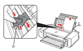
When the **Print Head Alignment** screen appears, load two sheets of A4 or Letter-sized plain paper in the Rear Tray (C) as shown.
