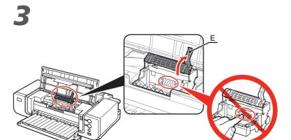
Firmly raise the Print Head Lock Lever (E) until it stops.
