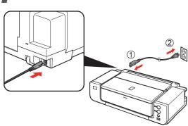
Plug the power cord into the back left of the printer, then connect the other end to the wall outlet.
