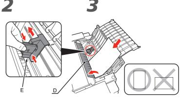
Open the Feed Slot Cover (D), then pinch and slide the Paper Guide (E).
