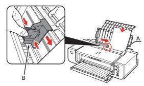
When the **Print Head Alignment** screen appears, load two sheets of A4 or Letter-sized plain paper in the Rear Tray (A) as shown.
