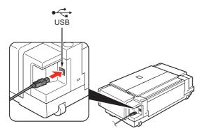
When the **Printer Connection** screen appears, connect the printer to the computer with a USB cable.
