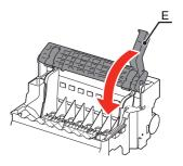
Lower the Print Head Lock Lever (E) completely.
