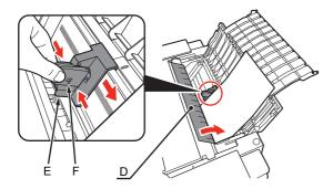
Pinch and slide the Paper Guide (E) against the left edge of the paper, then close the Feed Slot Cover (D).
